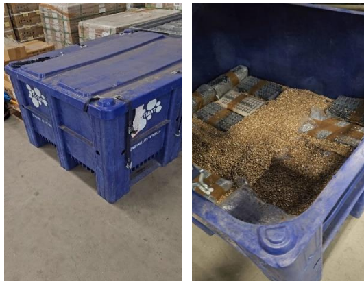
Figure 7 Special waste li-ion battery container for temporary storage containing Vermiculite prior transport by Stibat (at Cleantron Facility)
